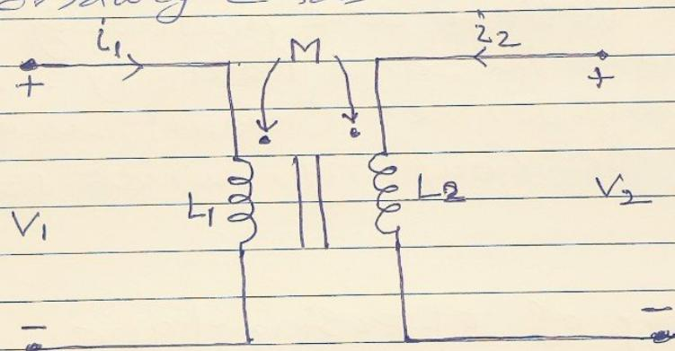
The currents flowing through Primary and Secondary coils are  $i_1$  and  $i_2$  respectively. In this case, these currents enter at the dotted terminals of respective coil. Hence, the induced voltage in each coil will be having positive polarity at the dotted terminal due to the current flowing in another coil.
