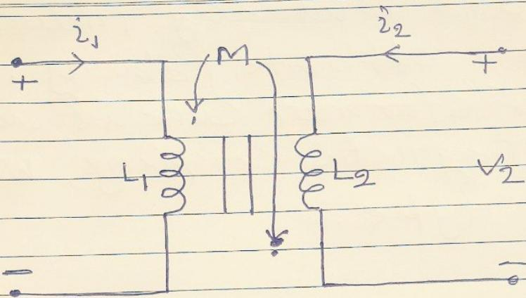
So positive polarity of the induced voltage is present at the dotted terminal of this Secondary coil.
